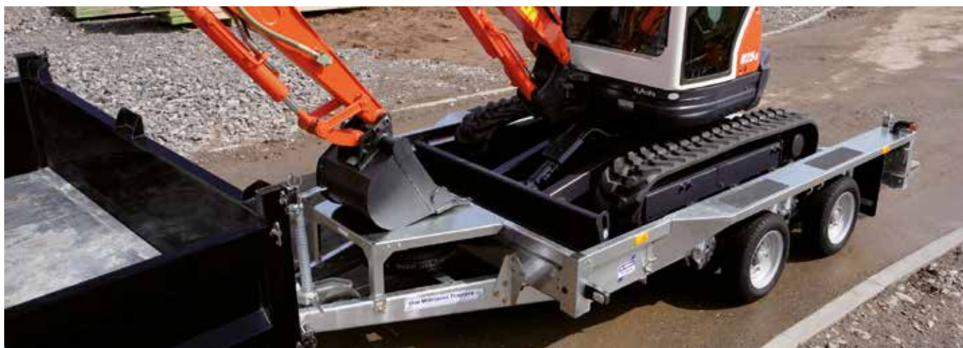
GX106 with skids and integrated rear supports
